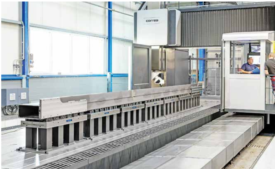
With the MAGNOS MFRS magnetic chucks, it is possible to clamp long welded assemblies with minimum distortion. This ensures perfect processing quality.
