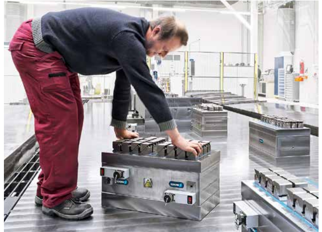
As soon as the lower magnetic chuck is deactivated, the machine operator can effortlessly move the clamping block by hand Image: SCHUNK
