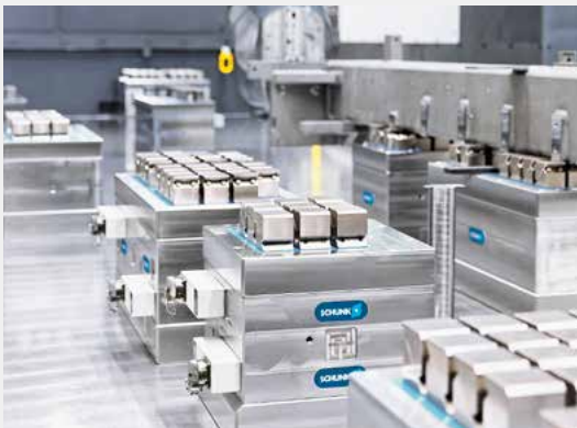
The machine table is completely covered with a steel plate and surface-milled. On this mirror-finish surface, the clamping modules can be very easily positioned. The ideal distance of the clamping blocks was trialed in a series of tests.
