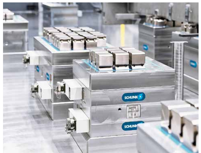
The machine table is completely covered with a steel plate and surface-milled. On this mirror-finish surface, the clamping modules can be very easily positioned. The ideal distance of the double magnets was tried in series of tests. Image: SCHUNK
