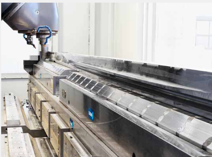
In order to compensate for heat distortion, the square profiles are clamped both on the foot and laterally by magnet. Three set-ups are sufficient to fully process the lugs.
