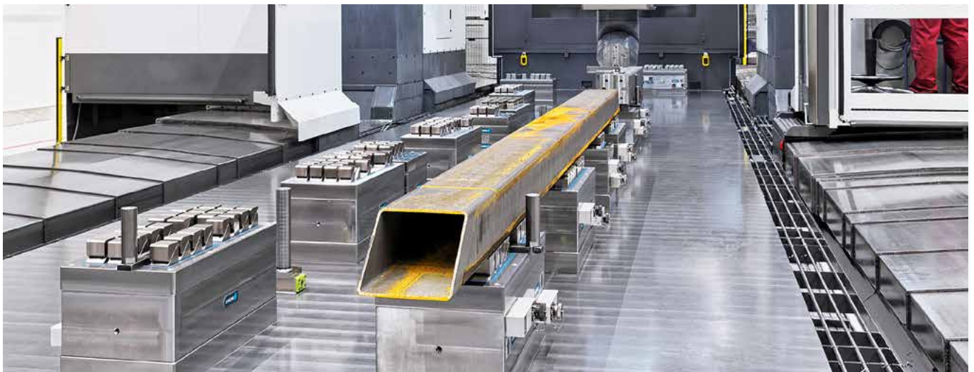
With the help of the SCHUNK magnetic solution, large-format welded constructions of up to 12,000 mm can be processed on a Correa OX M gantry type milling machine. Image: SCHUNK
