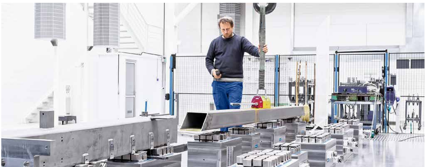
Since the machine table is free of grooves and holes, it is very easy to clean. Once the clamping modules are positioned, the pipes and welding frames are placed on the MAGNOS clamping modules by crane and clamped. Image: SCHUNK
