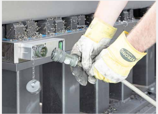
Patented status display: "Green" indicates magnetization status. Now the workpiece is firmly clamped to this magnetic clamping module. Image: SCHUNK
