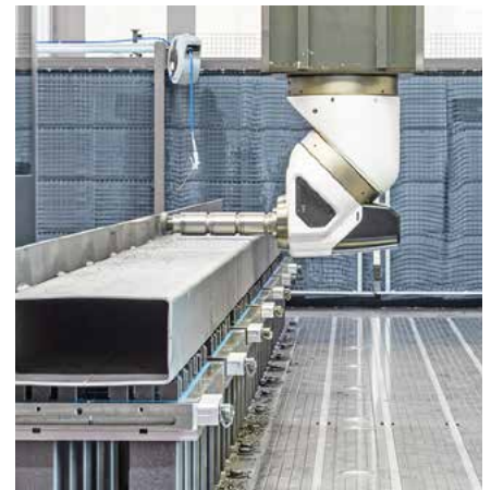
With the MAGNOS MFRS magnetic chucks, it is possible to clamp long welded assemblies with minimum distortion. This ensures perfect processing quality.
