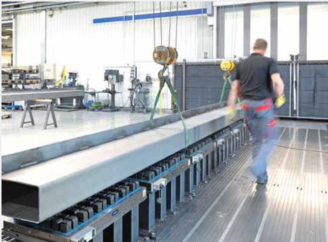
Thanks to the exemplary cable management, employees can move around the machine safely and without tripping hazards Image: SCHUNK
