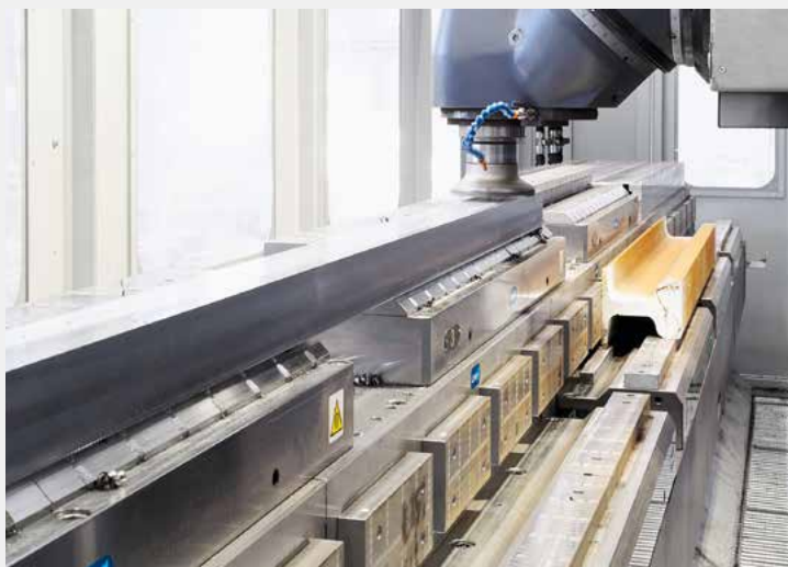
Before groove milling, the track elements are processed with the face-milling cutter. The workpieces are clamped on the foot and on the side on the rail head.
