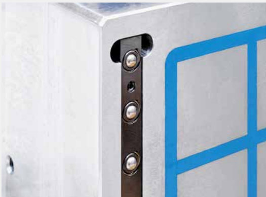
The roller block rails on the bottom make it very easy to position the clamping blocks when deactivated. As soon as the magnetic chuck is activated, the clamping block is securely clamped on the machine table.
