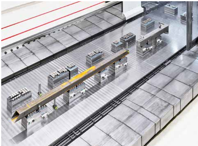
The machine table of the gantry type milling machine measures 12,500 mm x 3,000 mm. A partition wall allows machining in shuttle operation Image: SCHUNK
